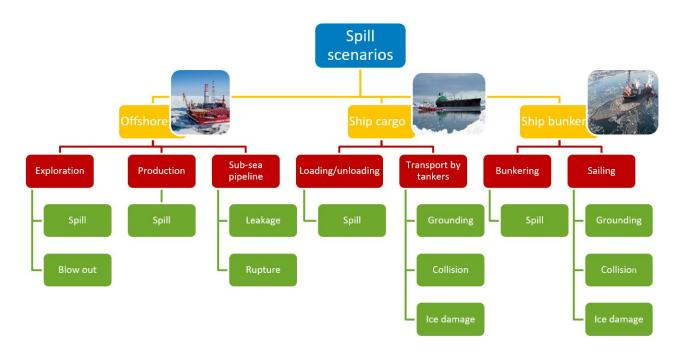
Figure 8. Various sources of potential oil spill and discharges in Arctic areas.
